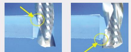
• Negative shear angle for clean edge on the top side
